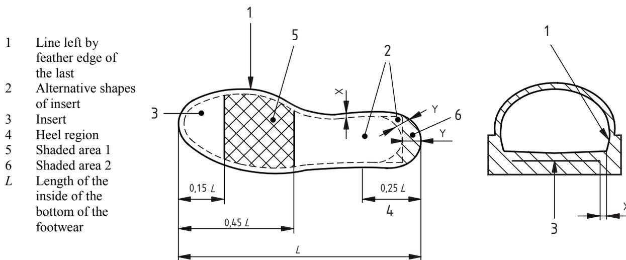
Figure 14 — Determination of dimensions for the insert
