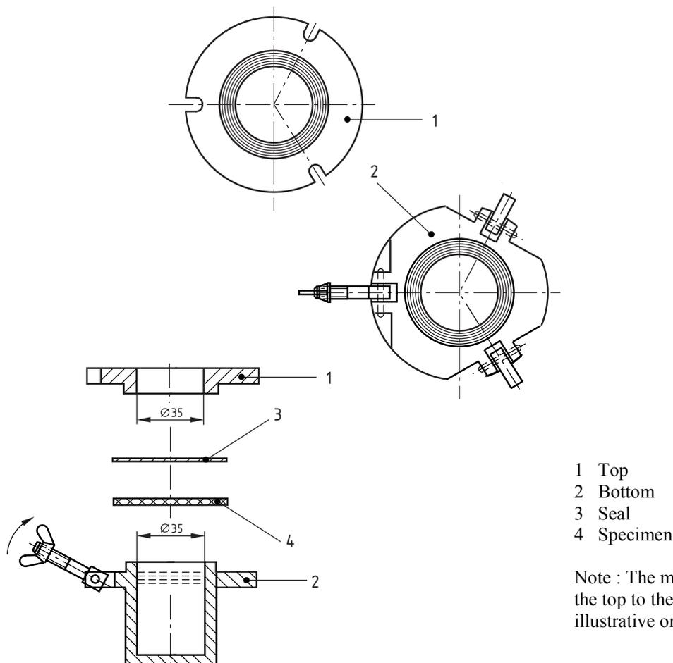
**Figure 39 — Apparatus for determination of W.V.A.**
