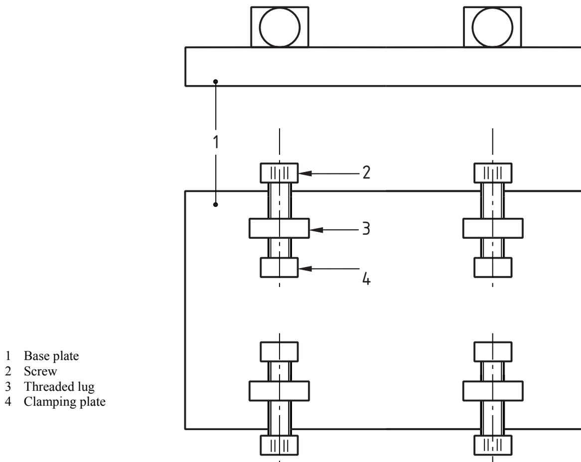
Figure 28 — Clamping device
