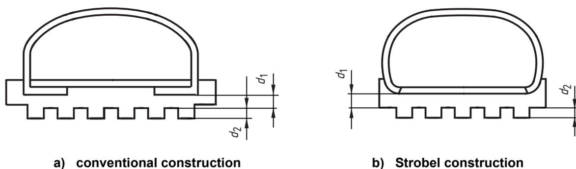
Figure 42 — Direct injected, vulcanised and cemented outsoles
