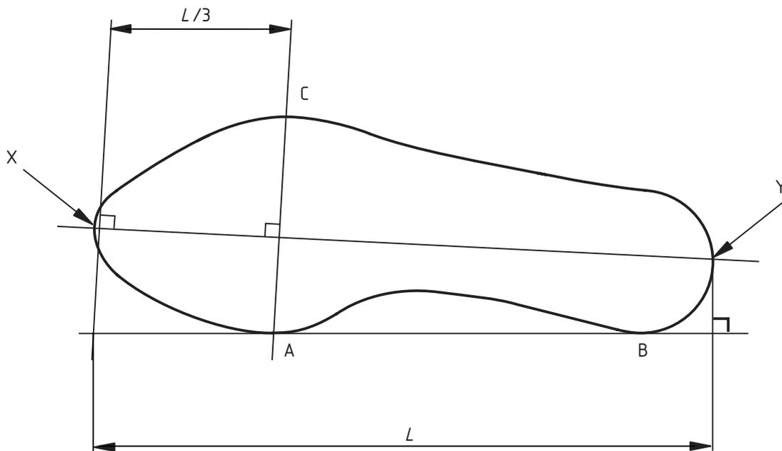
Figure 45 — Position of flexing line on the sole
