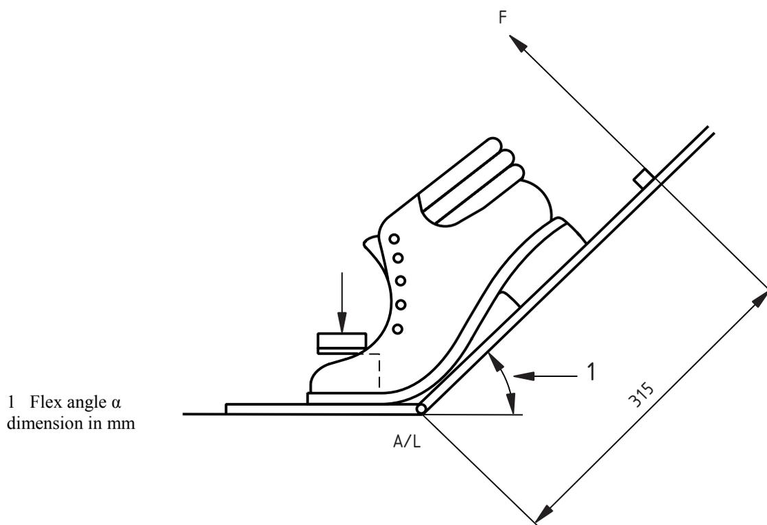
Figure 47 — Flexing angle
