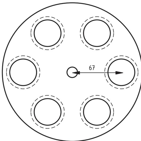
Figure 35 — Holder for jars used in WVP test
