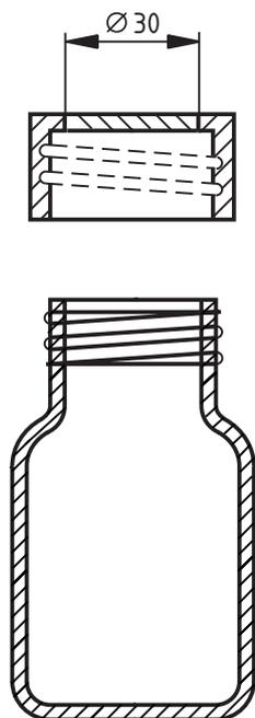
Figure 34 — Jar to be used in WVP test
