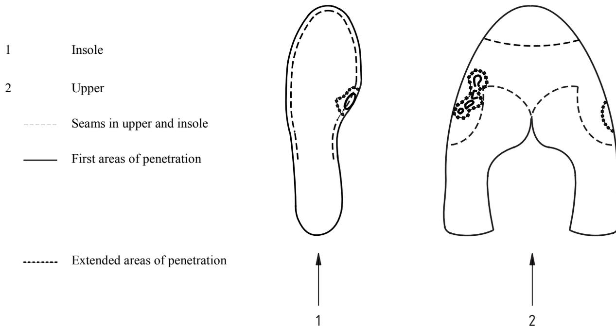
**Figure 21 — Suitable form of diagram for a shoe, with an example of recorded penetration added**
