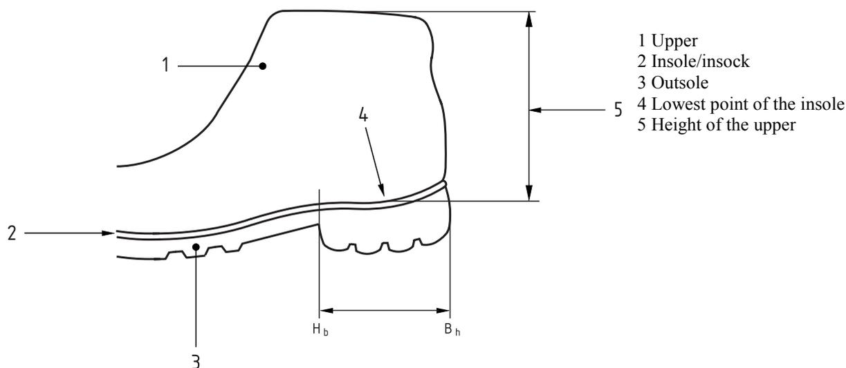
Figure 33 — Measurement of the height of the upper
