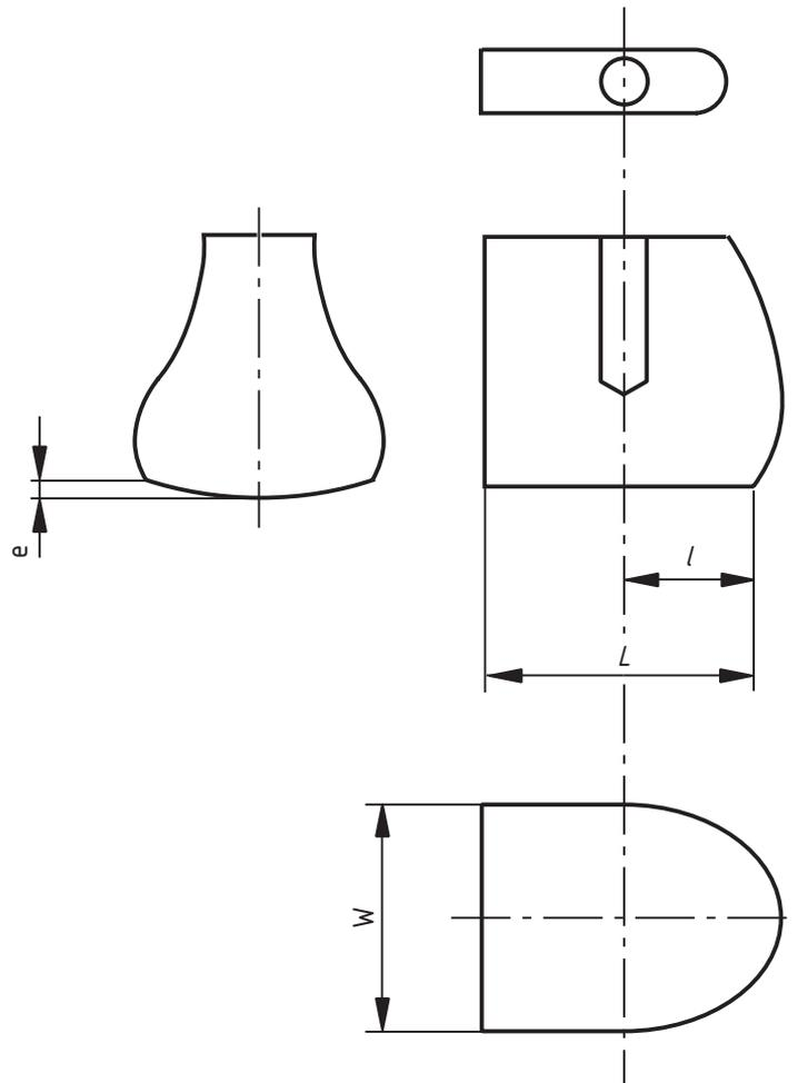
Figure 19 — Test punch for energy absorption test
